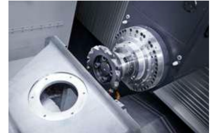
A WIDE RANGE OF ELECTROSPINDLES AVAILABLE The program offers a large variety of spindles available, to cover from high dynamics machinings to works on the hardest materials by high torque spindles.
