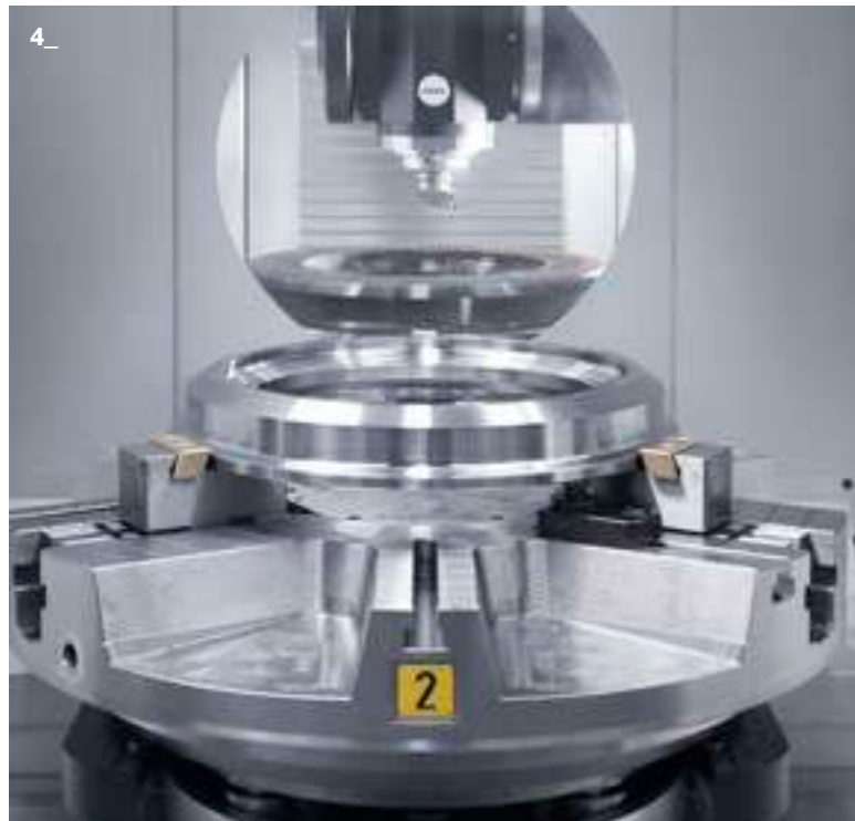
3_ THR 16 MULTIPROCESS with universal B-axis head (-15°/+195°). This multitasking machining centre has been adapted to the customer's needs, having increased the vertical travel by 300 mm, and is intended for the manufacture of different parts for the automotive sector.
